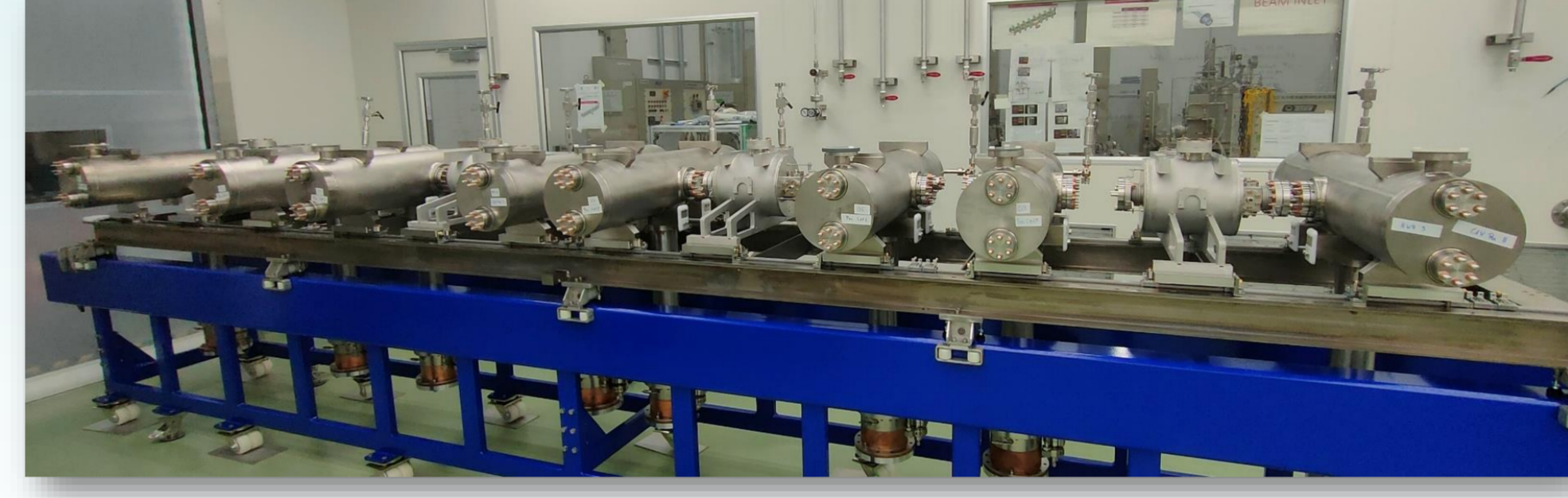
All 8 SRF cavities on the support frame
