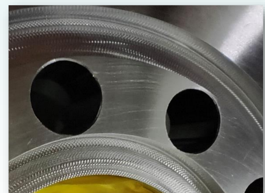
Sealing surface before and after repolishing
