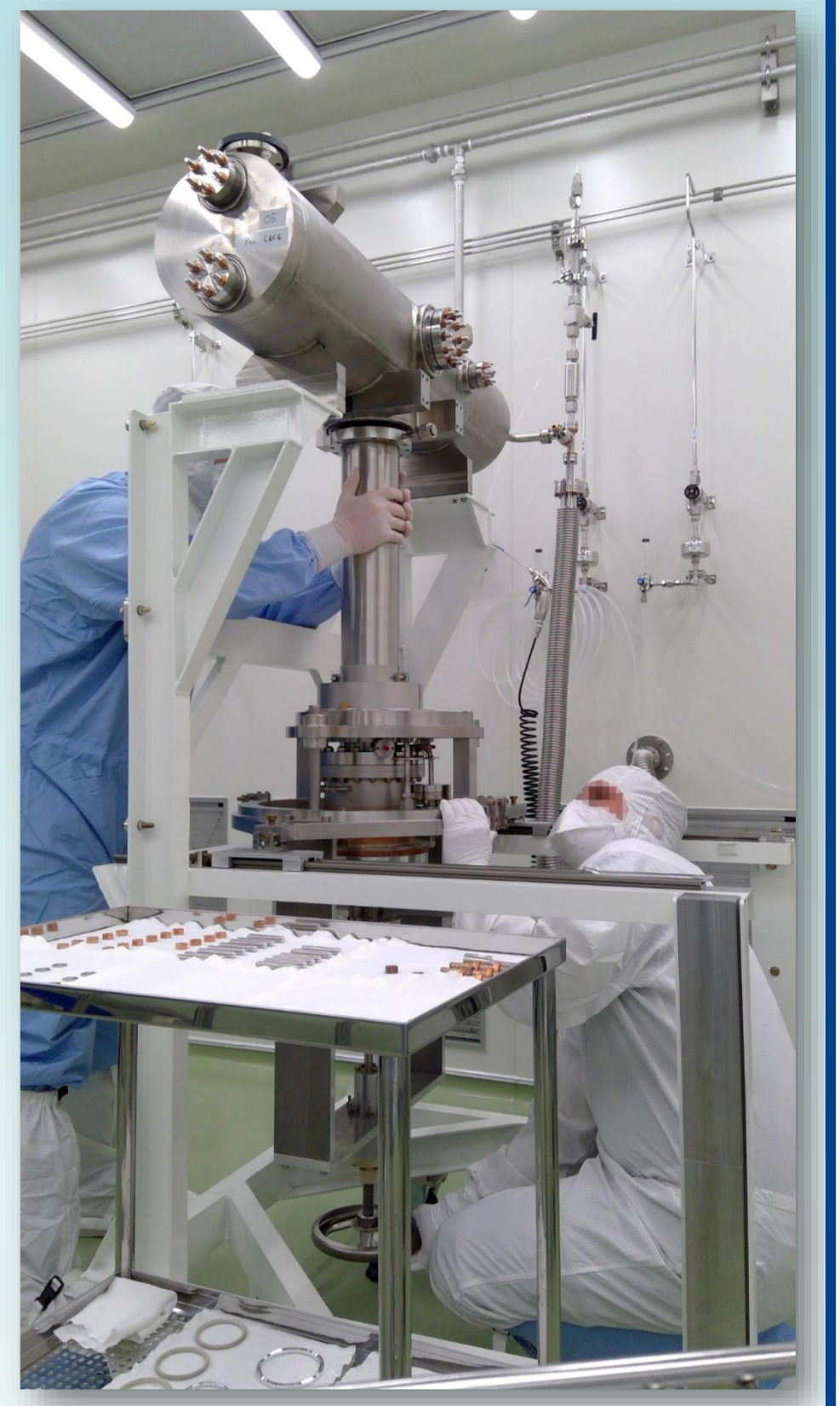
Cavity/Coupler Assembly Courtesy of RI GmbH
