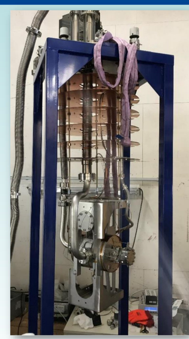
Solenoid on test insert
