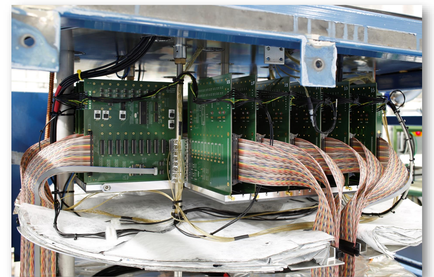
Sensor signals digitized inside of cryostat by custom-build evaluation boards to: extensively reduce number of feed-throughs, shorten analog signal lines and reduce thermal noise
