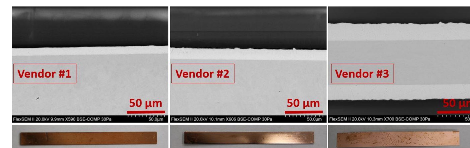
Cross section and thickness measurement from 3 plating vendors
