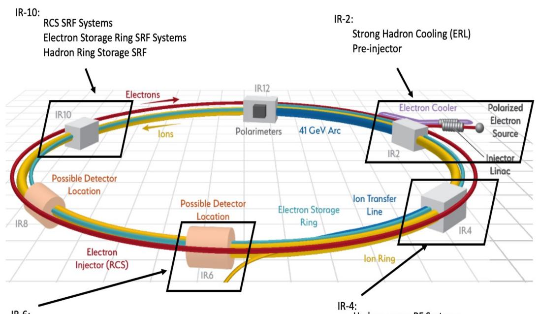
197 MHz and 394 MHz Hadron Crab Cavity Systems 394 MHz Electron Crab Cavity Systems
