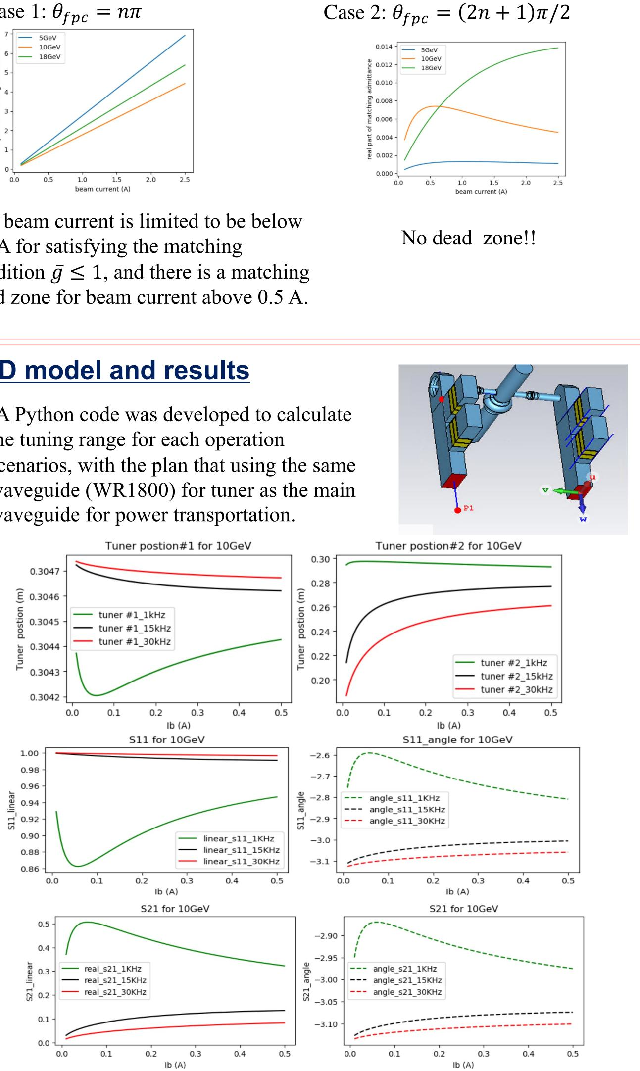
This paper describes the procedure to design a waveguide tuner for EIC eSR SRF cavity, so as to satisfy wide range of operating scenarios. The work is still ongoing.
