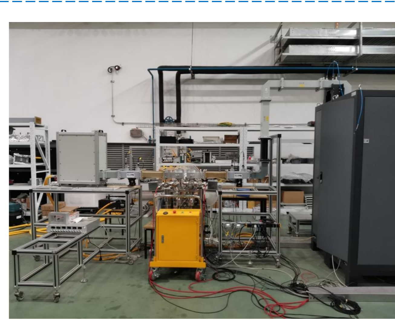
FIG. The layout of RF test system for 1.3 GHz FPCs
