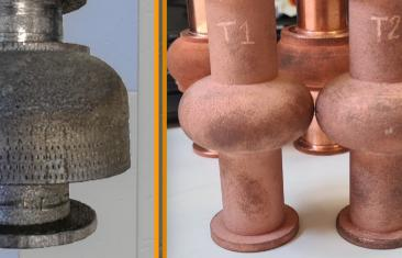
Nb "big cavity" Nb "small cavity" Cu cavity "T1" & "T2"
