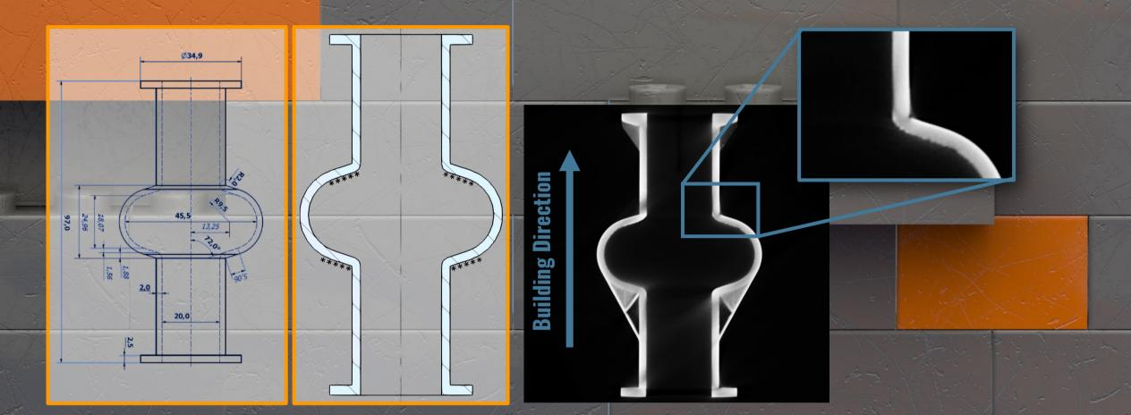
All cavities underwent RF resonance testing at room temperature, demonstrating excellent reproducibility. Leak tests were performed before and after each mechanical and chemical treatment. A sample Nb specimen, printed using Additive Manufacturing, was subjected to RRR (Residual Resistivity Ratio) testing at 300K and 10K, as well as critical temperature testing using the inductive method. The results showed an average frequency of 6 GHz (±0,14%), a Tc of 9.15 ± 0.1K, and an RRR of 8.
