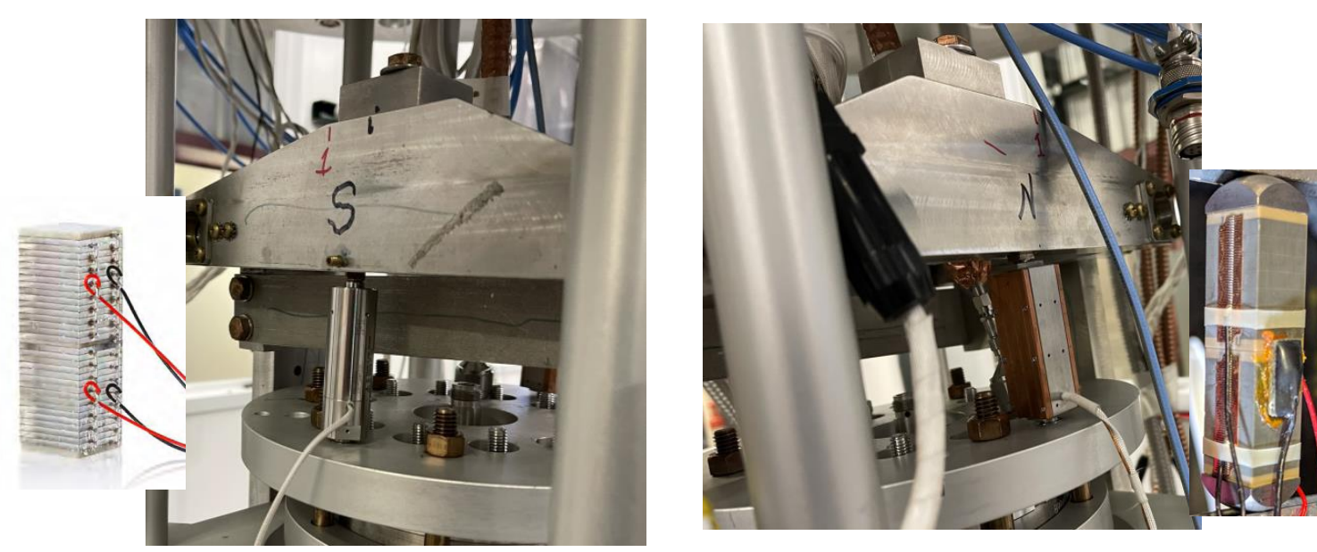
Figure 2: Close-up look at the location of the piezos on the cavity tuner. Left is the LiNbO 3 and right is the PZT.
