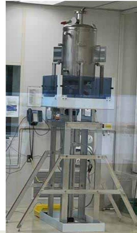
Rotational HPR with minimum numbers of water jets
