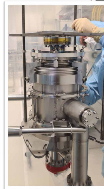
cavity ready for vertical test
