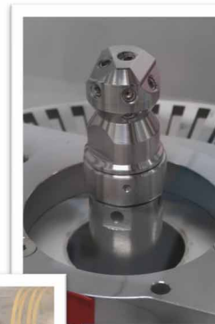
HPR with special gun nozzle
