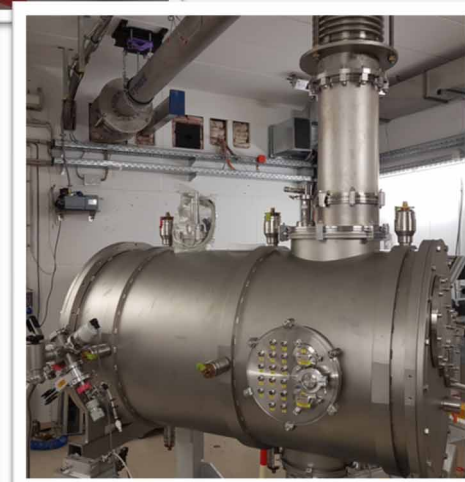
SRF gun III cold test in the bunker (w/o cavity)
