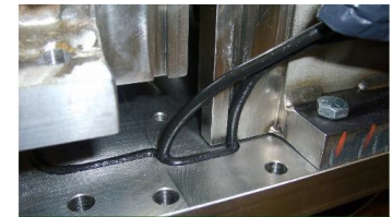
3 Way O-ring Separated Cavity/Cryomodule Isolation Vacuum
