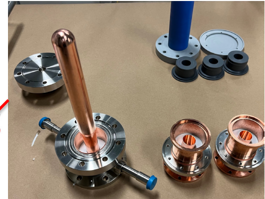
Fundamental Power Coupler
