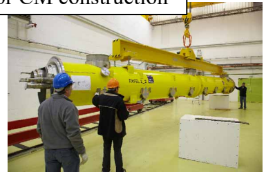
Hanger and rail system for CM construction
