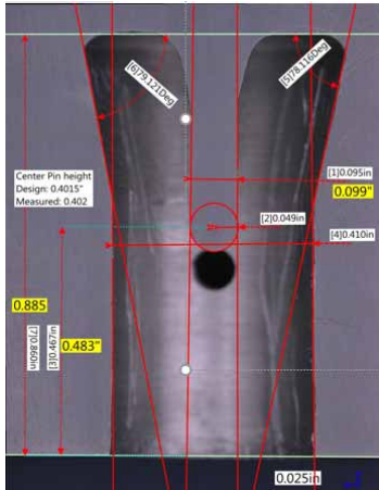
Dimensional analysis of part in cross section
