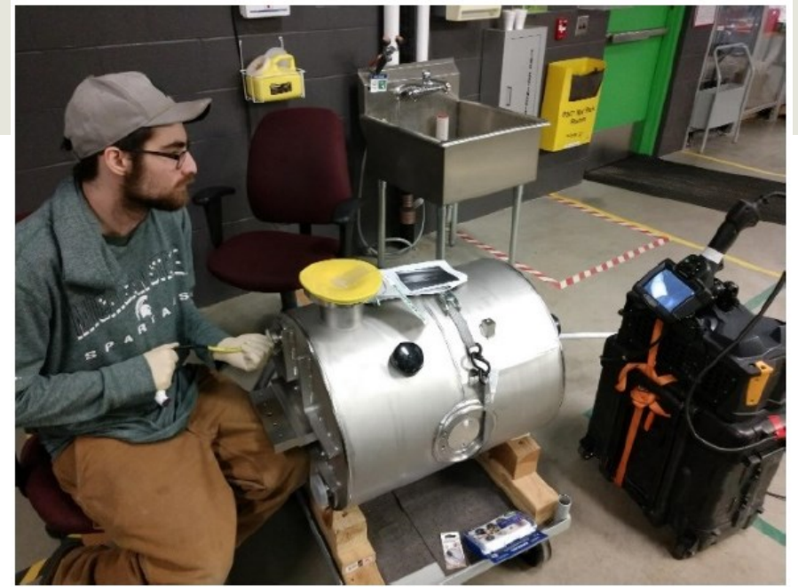
Figure 2: HWR polishing using the borescope (right) and a manual polishing tool (left).
