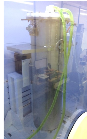
Chemical etching (BCP of \beta = 0.086 QWR)
