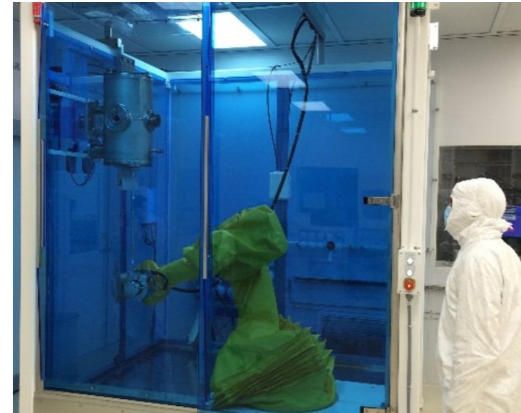
Rinsing: high-pressure ultra-pure water in clean room (HPWR of \beta = 0.29 HWR)
