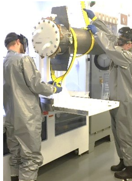
Chemical etching (BCP of \beta = 0.086 QWR)
