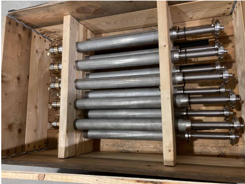
30 CV04 Valve stem dismantled
