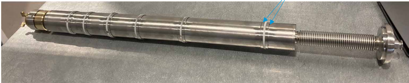
CV04 Valve stem modified
