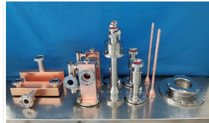
3.9GHz FPC prototype sub-assemblies
