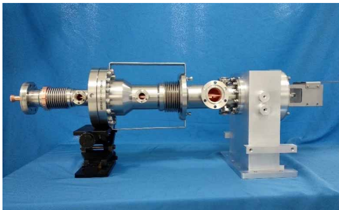
SHINE 1.3GHz FPC prototype
