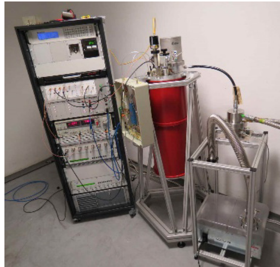
Cryostat (in red) for ultra-stable cryogenic clock developed by FEMTO-ST
