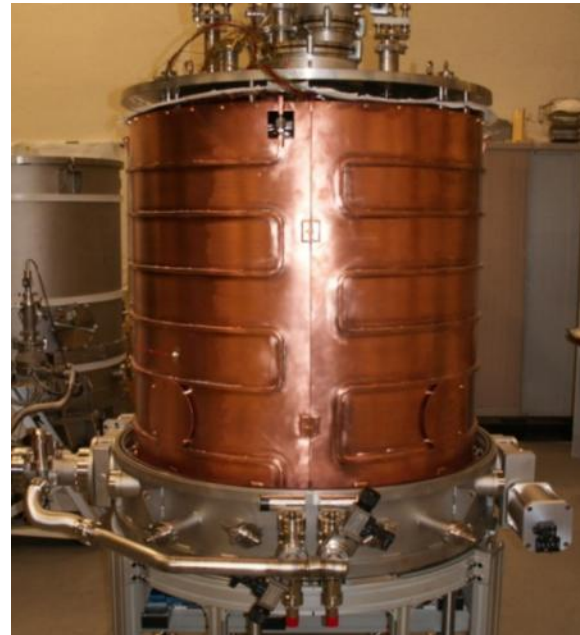
Thermal shield in copper with brazed pipes for cryogenic fluid
