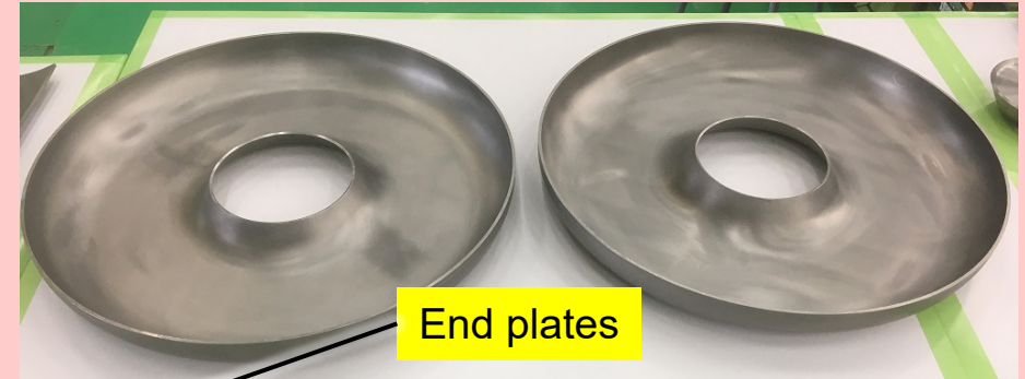
Press formed from Nb sheets (3.5 mm t)
