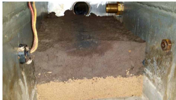
Decontamination cross section for a 10 MeV beam into a high-clay-content 5% contaminated soil
