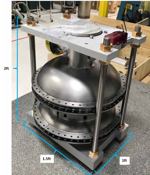
650 MHz Nb 3 Sn cavity (Cryoload ≈ 3.8 W @ 5 K)
