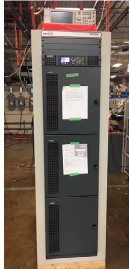
20 kW Solid State RF Amplifier
