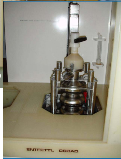
Ultrasonic cleaning tank at DESY (up to 1000L)
