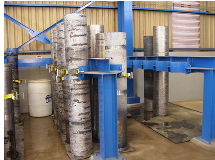
Electron beam melted ingots at CBMM
