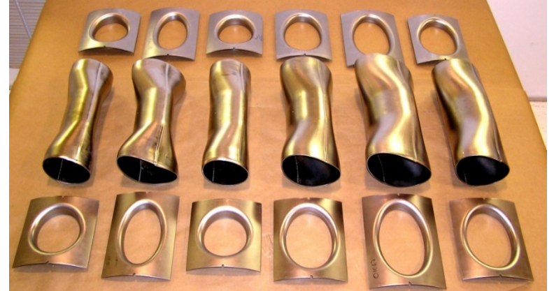
Cavity components prior to EBW (AES)
