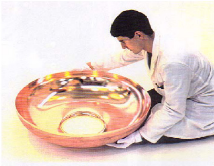
Copper half cell for LEP-II SC cavity
