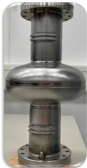
Single-cell 1.3 GHz SRF cavity
