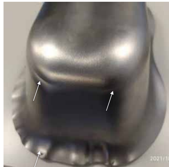
RFD pole forming trials for pre-series cavities, courtesy ZRI SRL.
