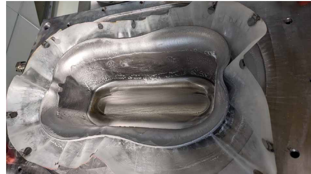
Preparation of the RFD Pole forming trials held at CERN Main Workshop EN-MME (May 2022).
