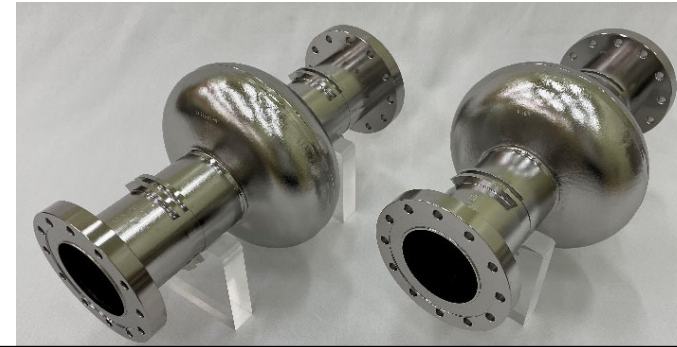
R18 & R18b HRRR MG Nb Tesla cavity manufactured at KEK-CFF
