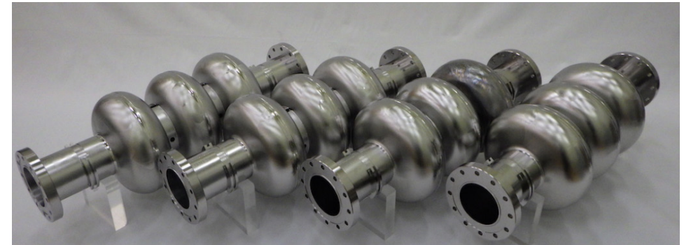
3-Cell LG Nb cavities manufactured at KEK-CFF
