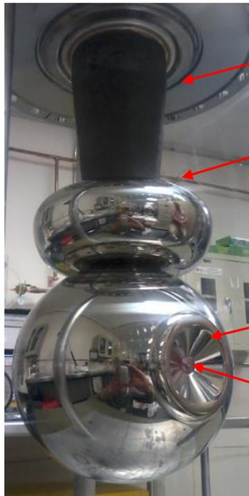
350 kV alumina insulator
