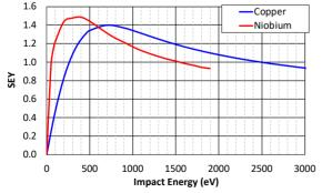
Figure 3: FEY curves for copper and Nb.
