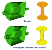
Figure 10: Minimizing the b3 and b5 multipole terms by introducing a curved pole profile.
