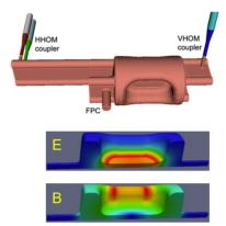
Figure 1: 197 MHz RFD cavity and field contour plots.
