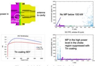
Figure 6: Multipacting in FPC window.
