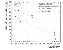
Figure 4: Dependence of the critical temperature of the Nb<sub>3</sub>Sn films on the cathode power. The films on sapphire substrate show trends with cathode power, coating pressure and coating temperature.
