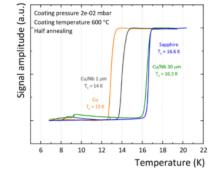
Figure 5: Superconducting transition curves of samples deposited at 600 °C. The Nb<sub>3</sub>Sn coated onto a thick Nb barrier layer shows same Tc as sapphire substrate ones.
