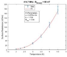
Figure 10: QPR sample RF test after optimized metallographic polishing. Rres value better than 1 n $\Omega$  demonstrate that QPR is now able to measure R\_res with same accuracy and precision as an SRF cavity.
