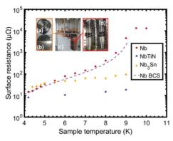
Figure 9: An example of surface resistance as a function of temperature for a planar Nb/Cu and NbTiN/Cu samples. Inset: (a) the choke cavity, (b) Nb/Cu planar sample, (c) RF facility, (d) a split cavity.
