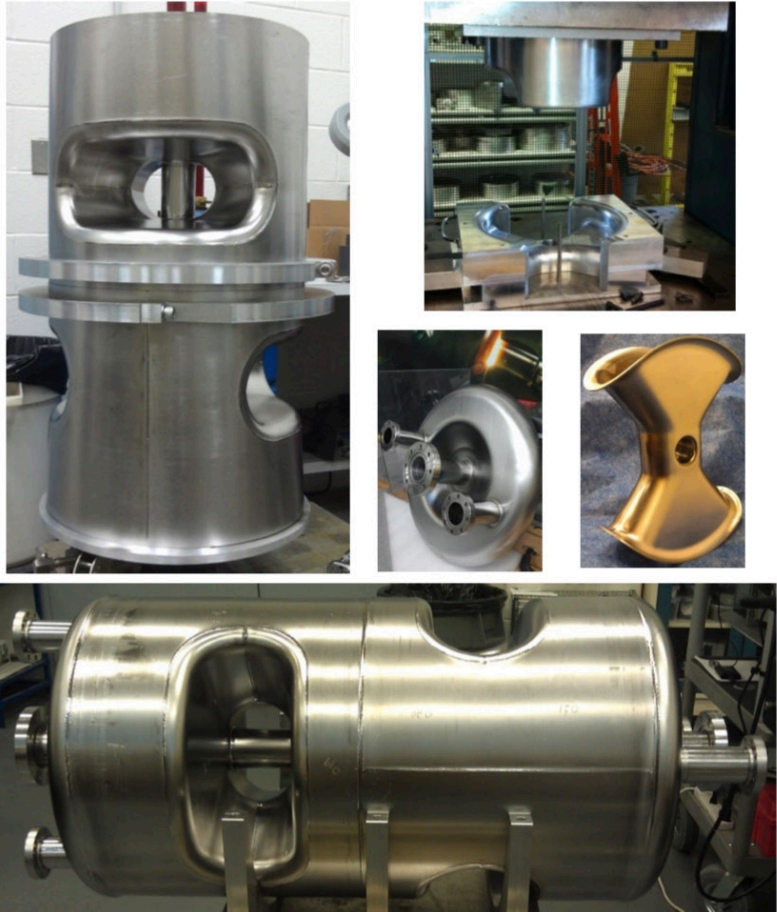
500 MHz Double-Spoke Fabricated at Jefferson Lab (HyeKyoung Park)
