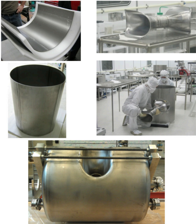
325 MHz Single-Spoke Fabricated at Niowave Inc.
