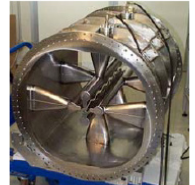
Superconducting RFQ Cavity
