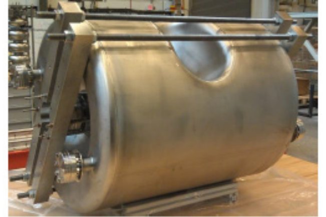
325 MHz \beta=0.82 Single Spoke Cavity
