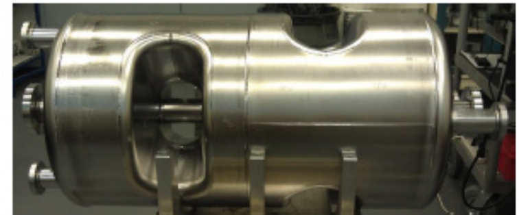
500 MHz \beta=1.0 Double Spoke Cavity
