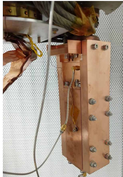
Split cavity mounted on the cold head for cryogenic measurements
