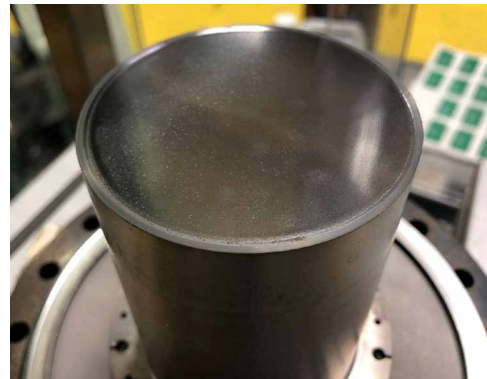
A QPR sample during and after the Nb deposition
