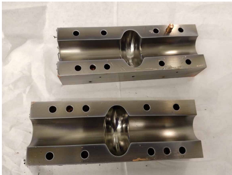
Nb thin films coated split cavity
