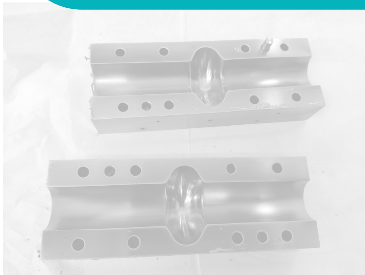
Nb thin films coated split cavity
