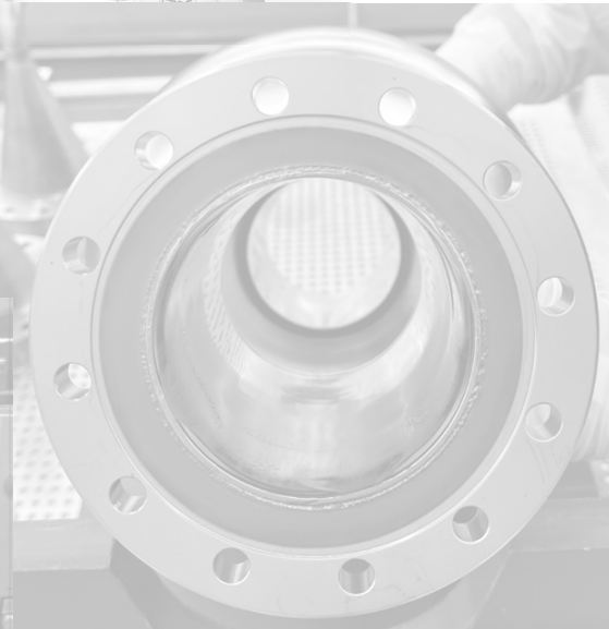
AIN-NbTiN coated cavity
