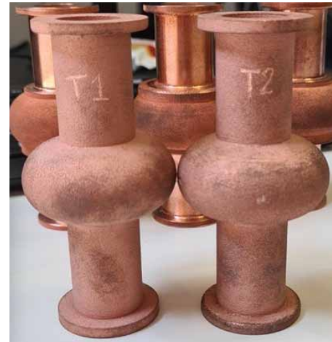
2 prototypes produced using TRUMPF TruPrint 5000
